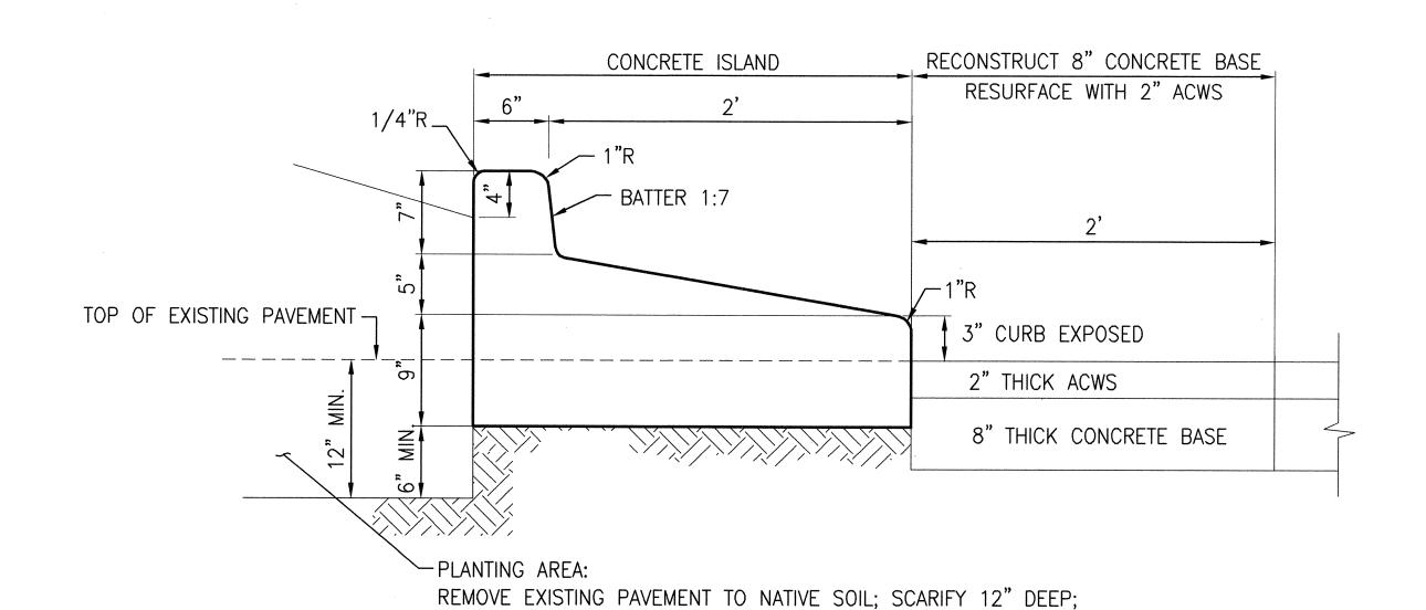
BACKFILL WITH TOPSOIL PLACED IN 9" MAX. LIFTS; COMPACT EACH LIFT WITH 200-LB GARDEN ROLLER;
