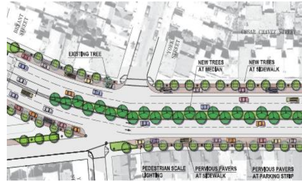
Center median with street trees
