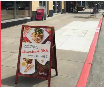
VIOLATION: A-frame signage is obstructing path of travel
