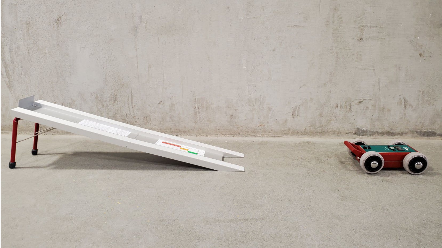
SlipAlert slip test equipment – correlated to ASTM E303-93 (2018).
