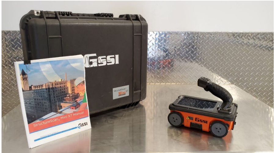
GPR Scanner (Ground Penetrating Radar)
