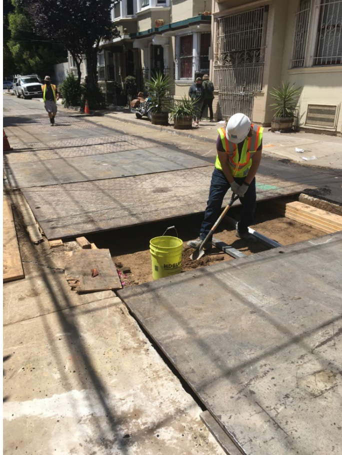
Grab sample of soil at field site for Moisture Density Curve and Sieve analysis.
