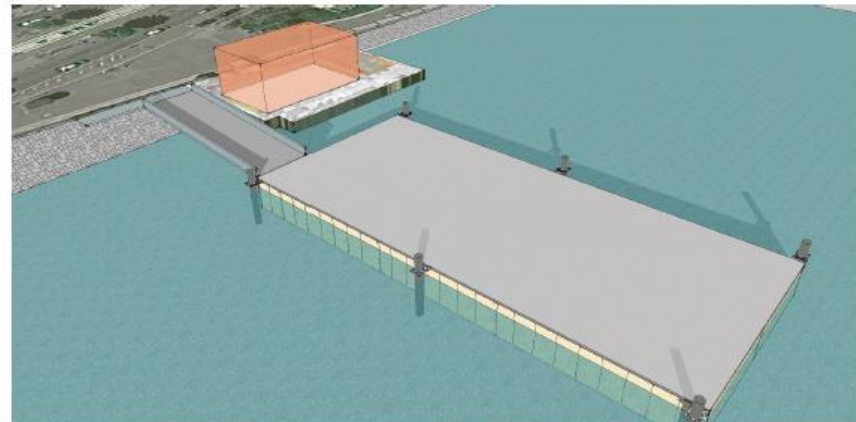
Steel Barge with Guide Piles and Ramp
